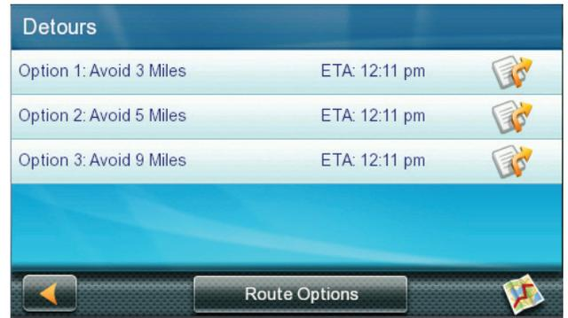
3. Different detours are calculated using the same routing method that was used to create the route. The list of alternate routes is displayed.
